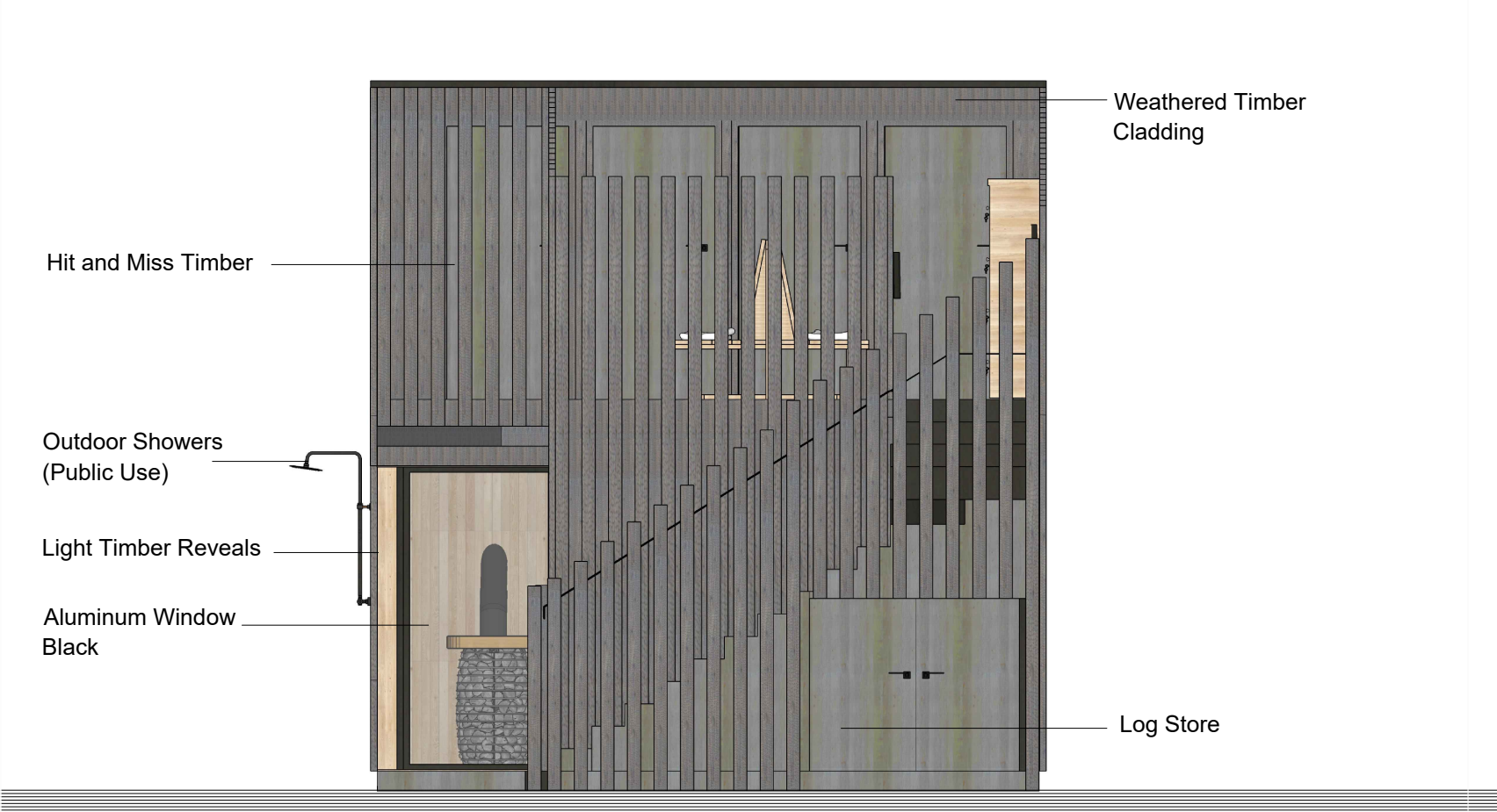
Proposed Sauna West Elevation Scale 1:50 @A1
