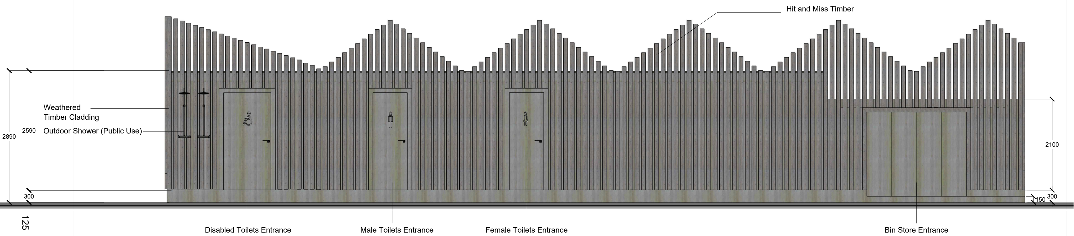
Proposed Toilets and Bin Store South Elevation Scale 1:50 @A1
