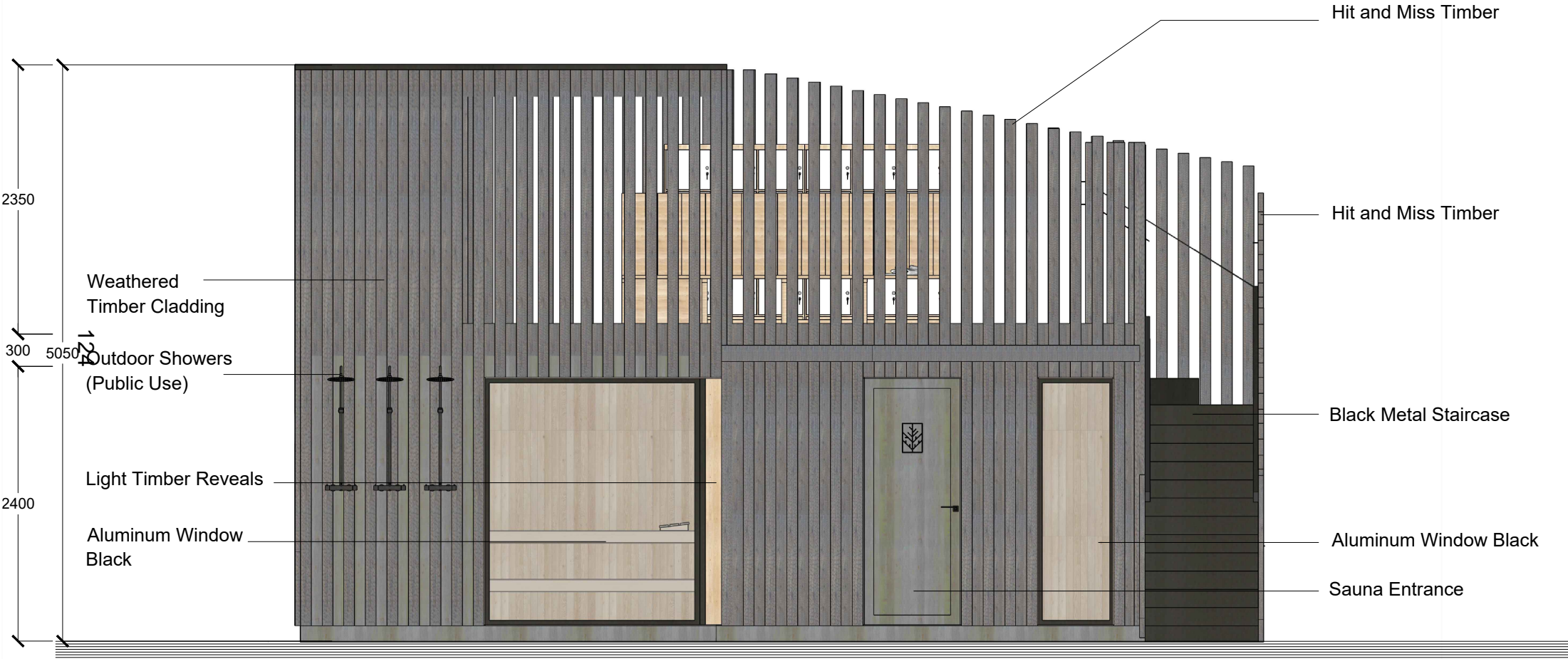
Proposed Sauna South Elevation Scale 1:50 @A1
